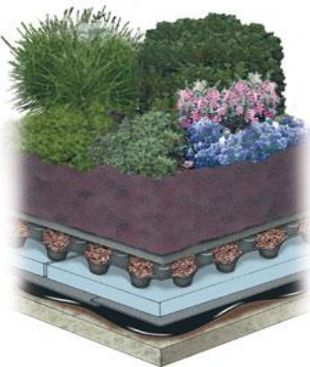
Figure 53: Intensive Green Roof System
