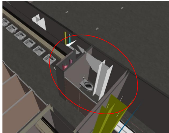
Figure 21: Structural vs. Architectural Clash
